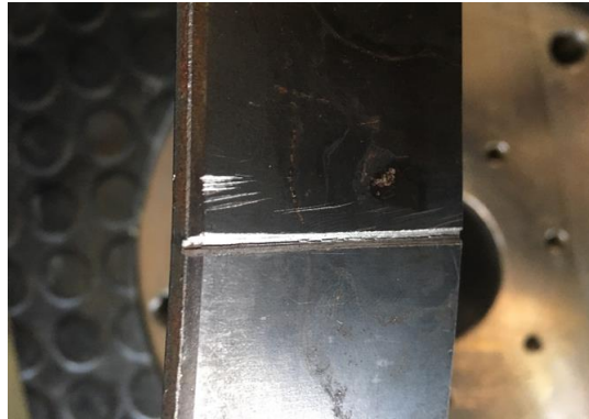
Fig. 7. A fatigue crack is well visible along the slit of the type 2 notched specimen.
